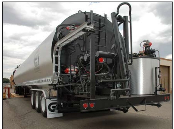
Additive system mounted on a portable asphalt tank.
